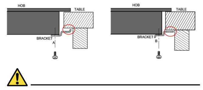
Under any circumstances, the brackets cannot touch with the inner surfaces of the worktop after installation (see picture).
