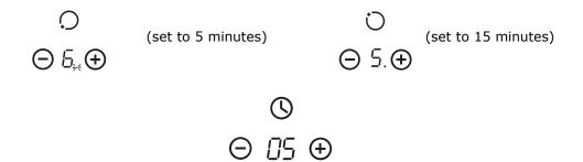
b). Once the countdown timer expires, the corresponding zone will switch off. Then it will show the new min. timer and the dot of corresponding zone will flash.
